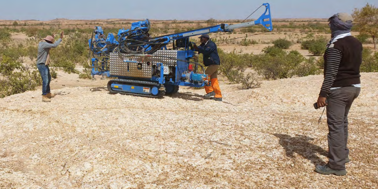
Preparations for borehole drilling to explore the kaolin deposit near Hassi Abyad in Mauritania.
