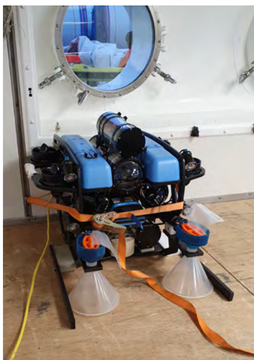
MARUM's ROV (BlueROV2) for sampling and observation of natural gas emissions in the North Sea.
