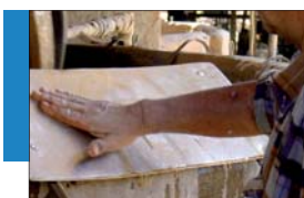
In the pan grinder, mercury is usually spread onto the amalgamation sheets with bare hands.
