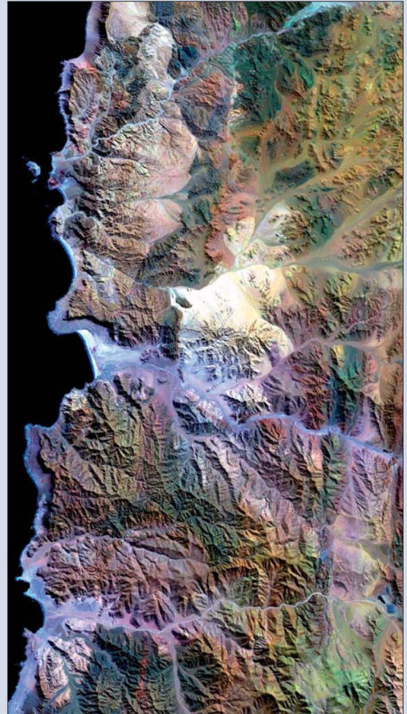
Flotation tailings of the Salvador copper mine belonging to the Chilean state mining company "Corporacion Nacional del Cobre de Chile" (CODELCO), located 1100 kilometres north of Santiago. Mine tailings which have been dumped into the sea for many decades have extended the shore line over a large area with partially contaminated material (satellite image: Landsat 7, BGR).
