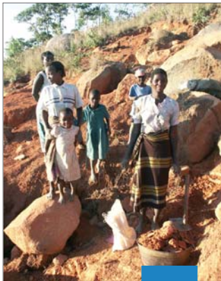
Extracting brick clay from a former debris flow on the west flank of Mt. Soche.
