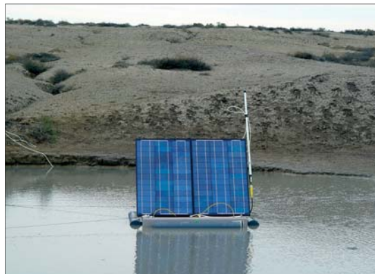
The BGR monitoring station on the Dashgil mud volcano collects gas rising up under a lake and records measurements including the change in the amount of gas upwelling over time.
