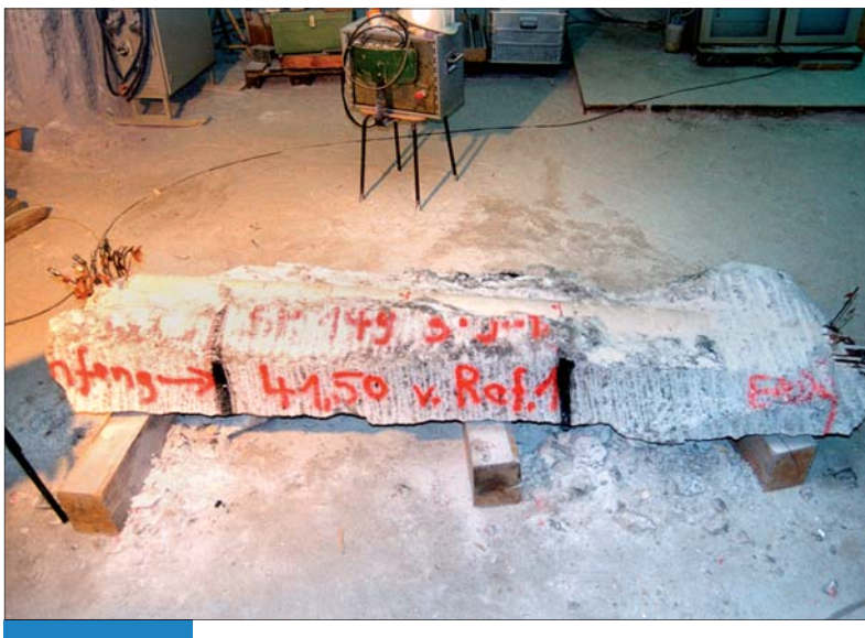
Exhumation of a stress monitoring station cemented into the salt for more than ten years.
