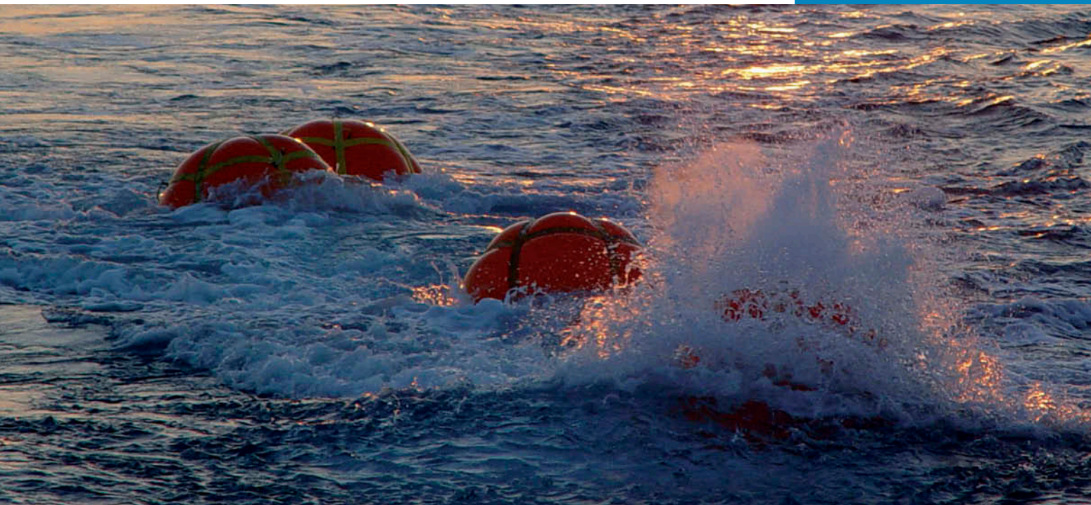
Air-gun shot generating seismic waves.
