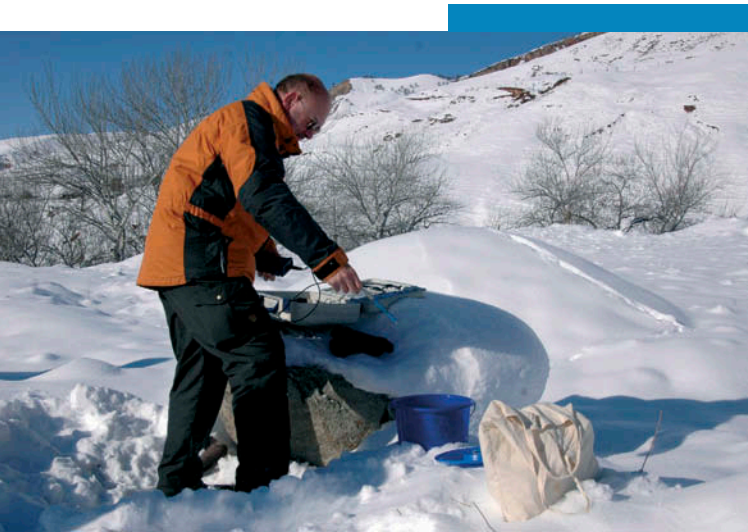
Analysing seepage water of a tailings pond near Mailuusuu using a mobile field laboratory.
