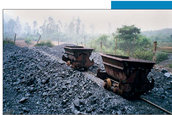
Operational safety risks: Unrestricted access to iron ore mine heap. Hand-operated trolleys are not secured against tampering.
