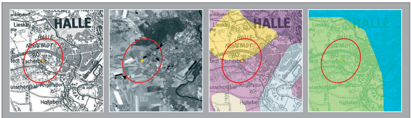
The automatically computed epicentre location (star) found by the ALISE system, together with the error ellipse (red) can be displayed on top of different maps. From left to right: topographic map 1:25.000; satellite image (25 m resolution); geological map 1:200.000. It can be superimposed with additional information like the area of potential damage (far right).
