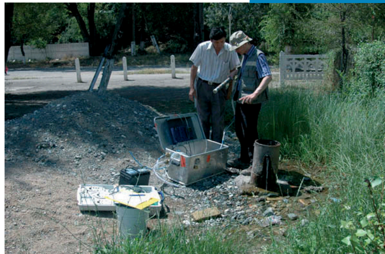
Water sampling and monitoring at an artesian well in Mailuusuu with mobile analytical equipment.
