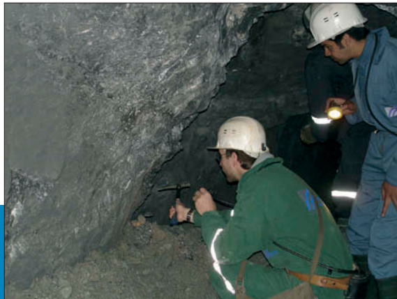
Sampling the cobalt ore in diorite the Bou-Azzer mine.
