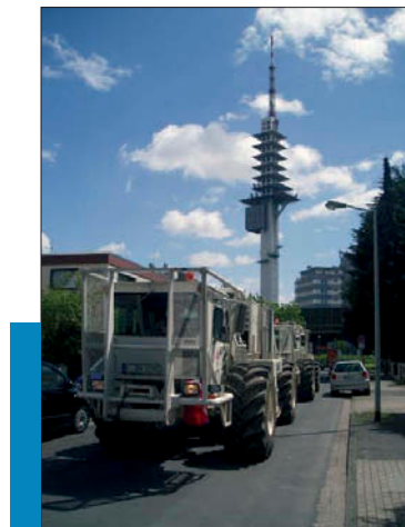
Shooting a seismic line using big vibration trucks operated by DMT, Essen, Germany
