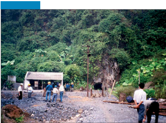
Hazardous: Unrestricted access to a working underground iron ore mine.
