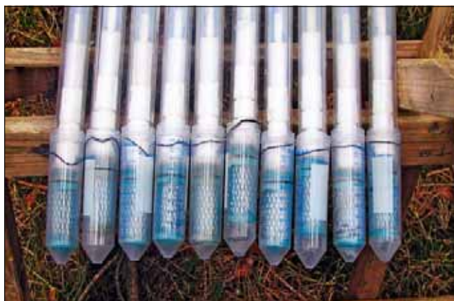
Ready for installation: the tips of percolation water suction probes.
