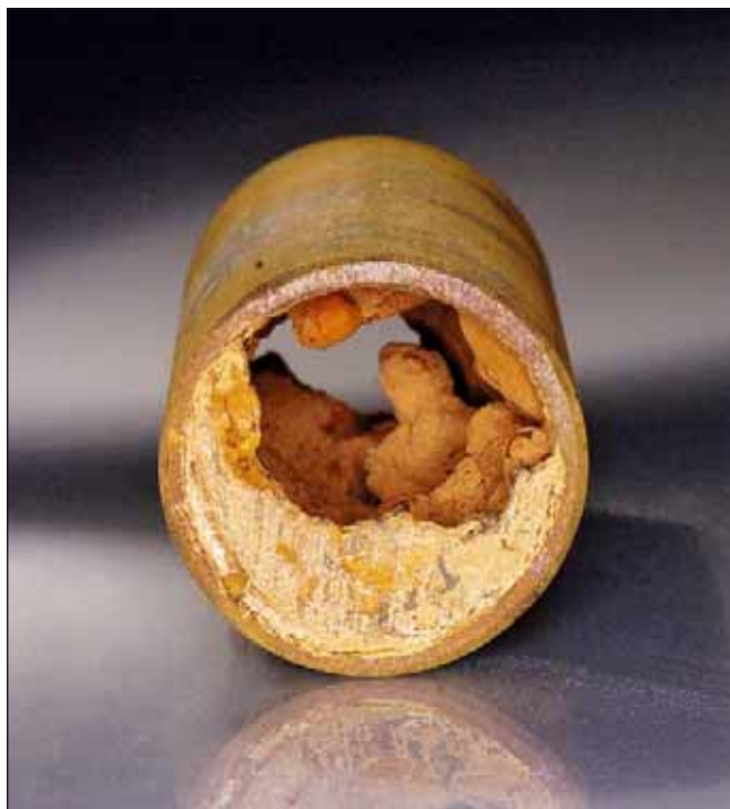
Pipe with encrustations.
