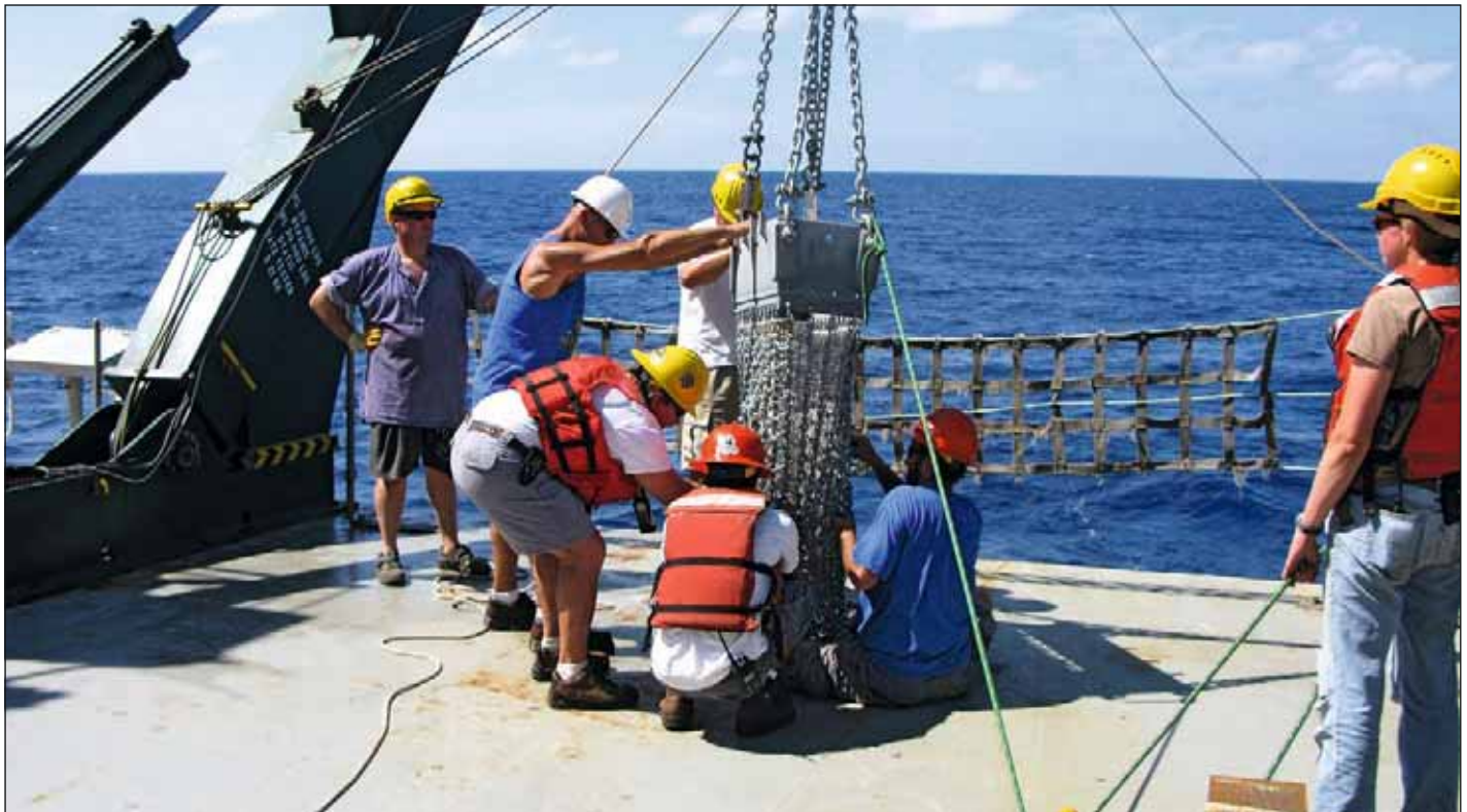
Preparing the deployment of a chain sack dredge on board of the 'Kilo Moana' research ship to extract a manganese nodule sample from a depth of 4,800 metres in the German concession.
