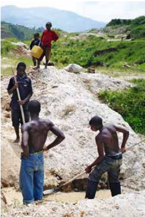
(left) Washing (ground sluicing) of the crude ore in preparation for pre-concentrate production.
