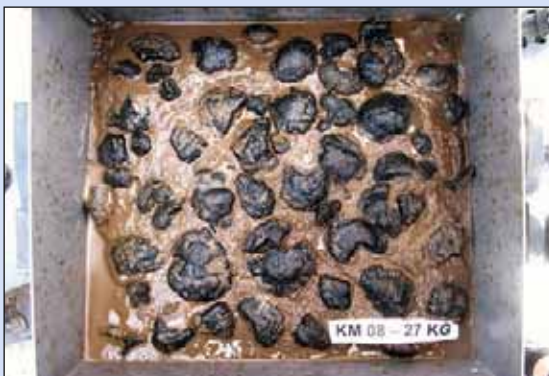
Top view of a recently recovered box corer. The box corer cuts out a small part of the seafloor measuring 50 x 50 cm including the manganese nodules lying on the surface, and brings the whole sample on board the ship. The nodules here measure around 5–10 cm in size and are often broken (irregular outline).
