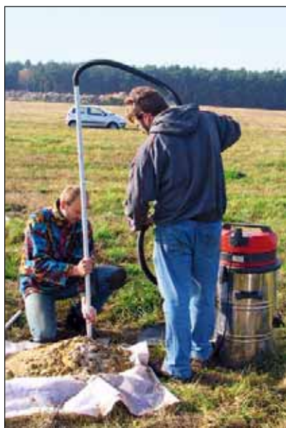
Preparing a borehole to extract a soil percolation water sample.
