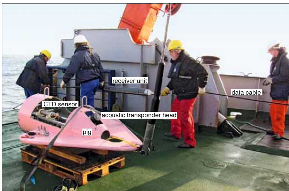
Deploying the CSEM system on the 'RV Poseidon' in the Black Sea. The receiver dipoles are attached to pressure cylinders housing the analogue electronics and the data loggers to record the signals.
