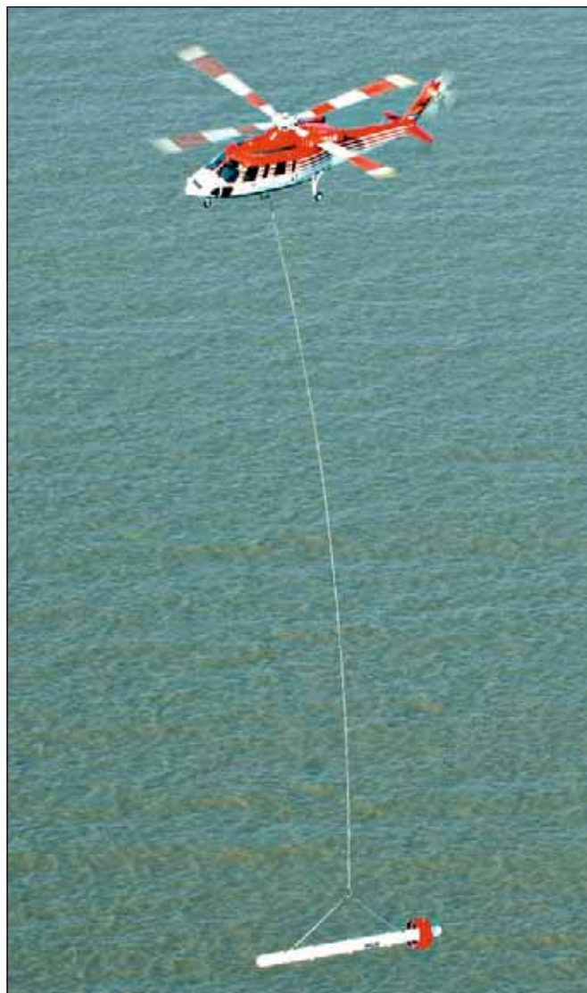
BGR helicopter towing an electromagnetic sensor over the North Sea.
