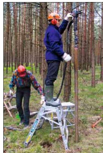
Extracting soil samples from the unsaturated soil zone down to the groundwater.
