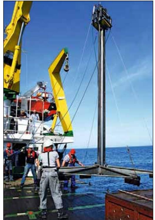
'Vibro-corer' to extract up to 6 metre long cores from the seafloor.
