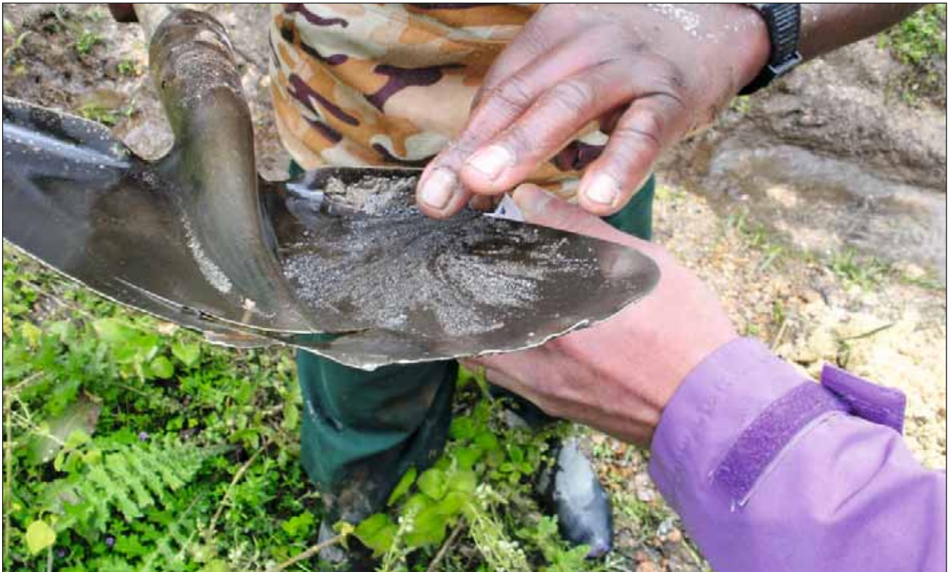
Sample extraction for the geochemical fingerprint of a coltan mine in Rwanda.
