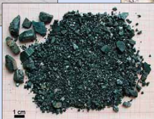
(upper left) Coltan washing site in Mozambique. (upper right) "Picking" – manually separating tantalite crystals from quartz, Ethiopia (below) Coltan ore from Brazil
