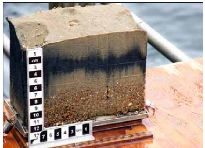
Box corer sample to determine the distribution of sediments on the seabed.
