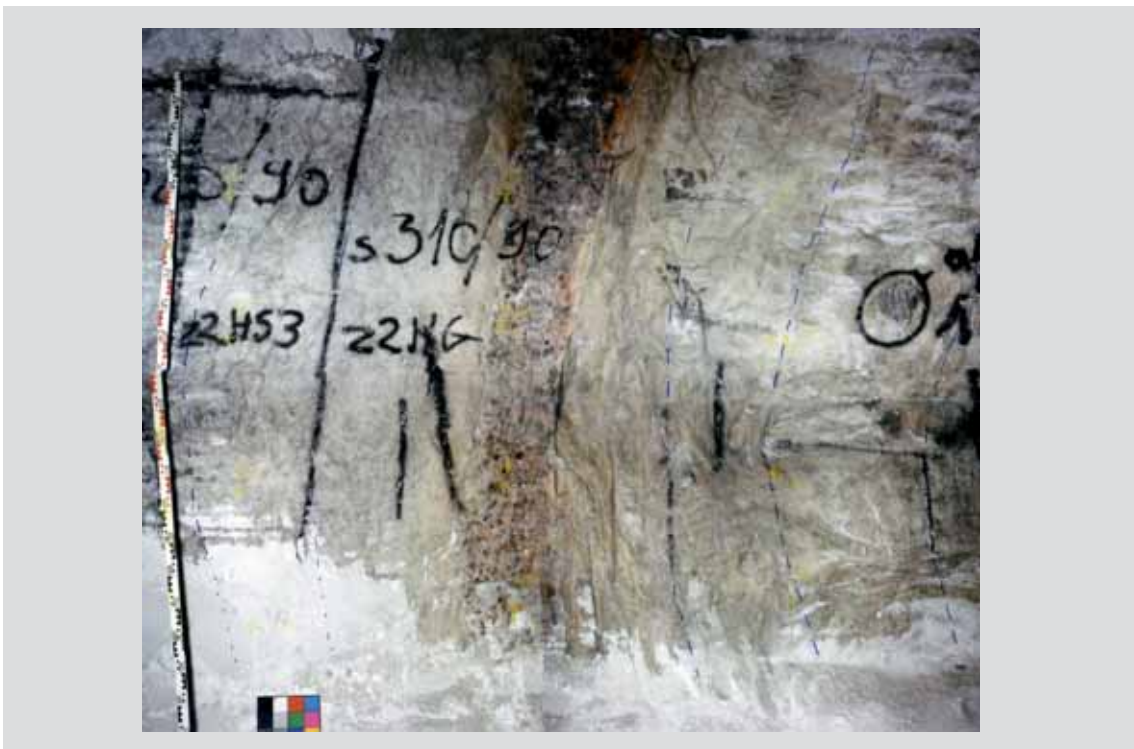
Figure 41: Boundary of Zechstein 2/Zechstein 3 with thinned-out Kaliflöz Stassfurt (centre) and halotectonic pinch-off of the sequence from Grauer Salzton to Hauptanhydrit (max. 100 m).
