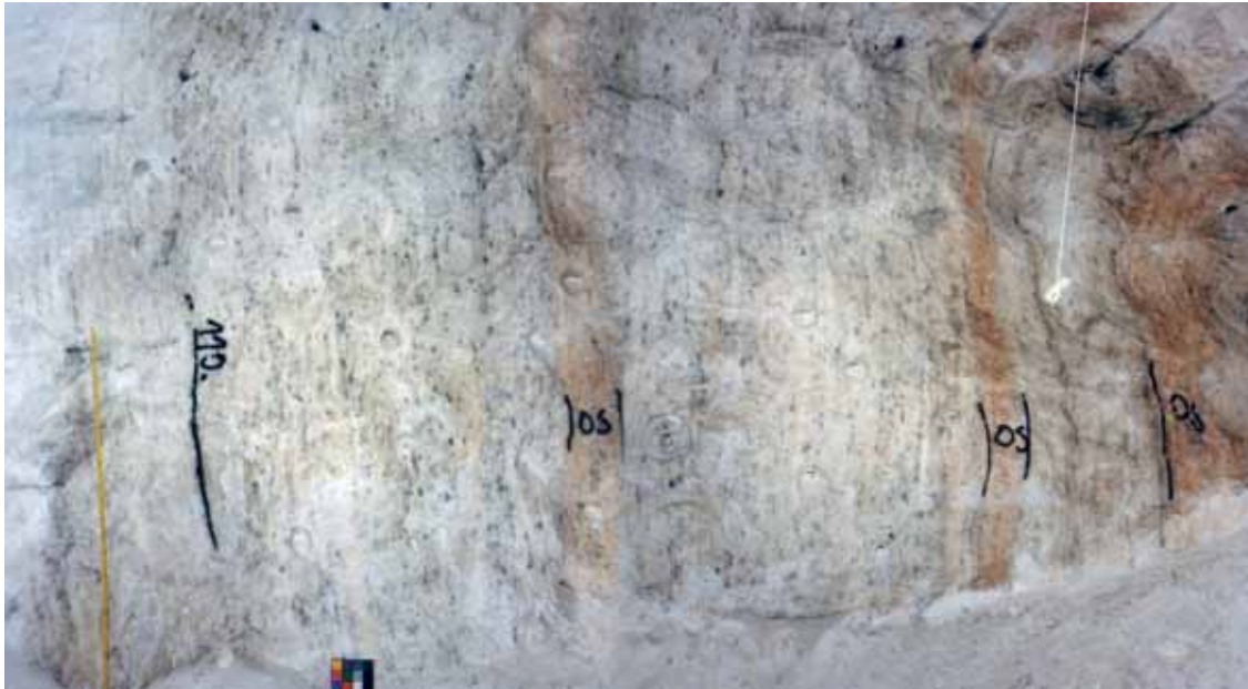
Figure 42: Intensely deformed and folded Liniensalz with isoclinal interfolding of Orangesalz close to the Zechstein 3/Zechstein 2 boundary. The stripe intervals are in the centimetre range and the anhydrite stripes are torn into segments. Shaft undercut to the 880 m-level, drift position 369 to 374 m, western wall. (Photograph: Bauer, DBE)
