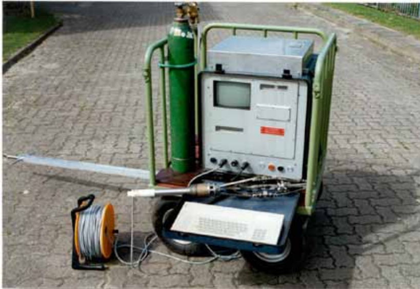
Figure 5.2: Temperature measuring apparatus in an ex-proof housing
