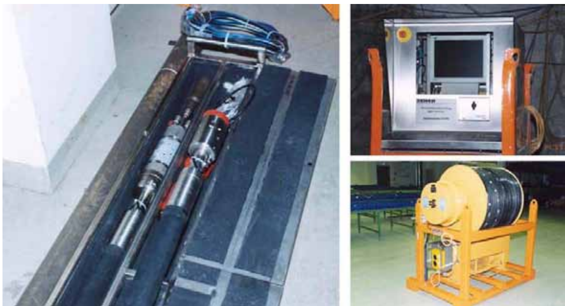
Figure 7.2: Permeability testing equipment (probe – data station – wireline cable)
