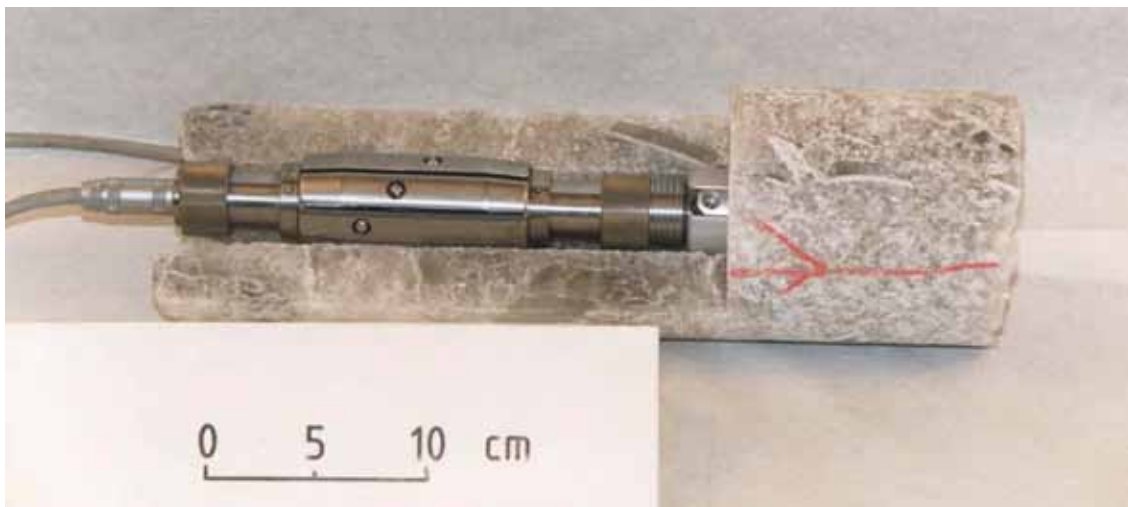
Figure 6.2: BGR overcoring probe type Mk14 in a rock salt core
