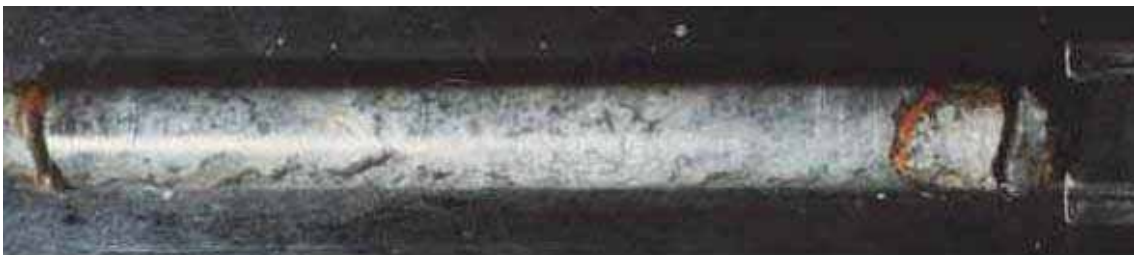
Figure 7.8: Core with healed joints in the Hauptanhydrit
