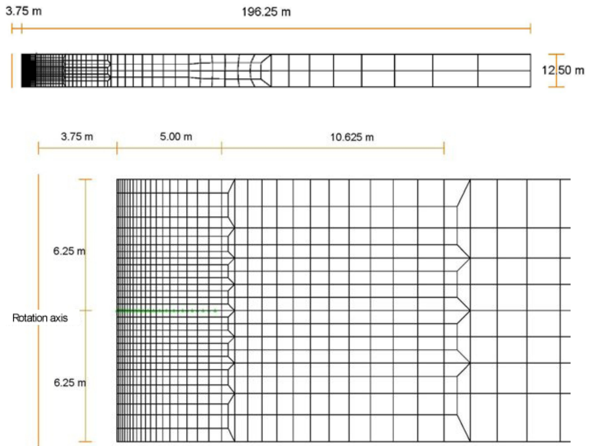
Figure 9.6: FE modelling of the shaft by an axi-symmetrical annular disc (above: total model; below: detail)
