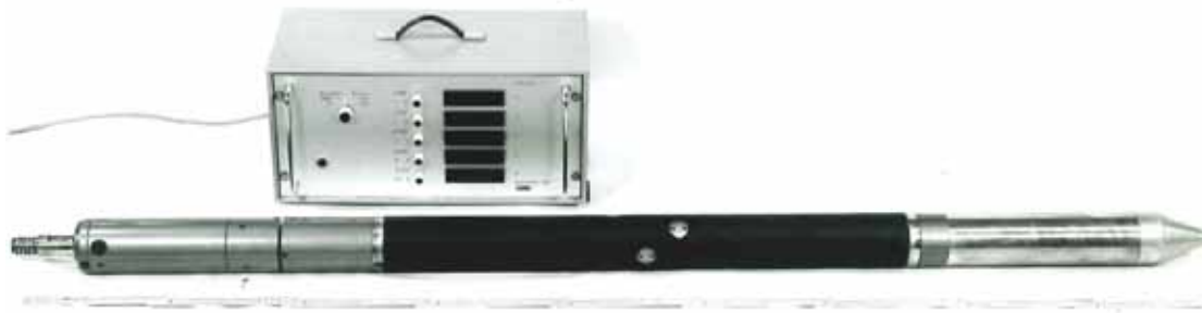
Figure 6.5: BGR dilatometer type Mk III
