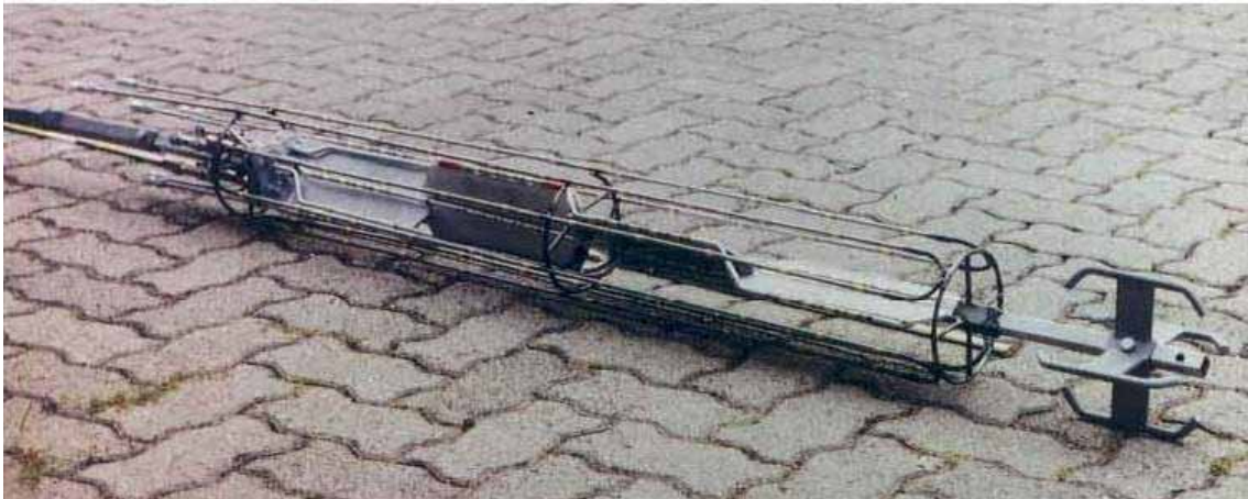
Figure 6.4: Stress monitoring stations with Glötzl pressure cells
