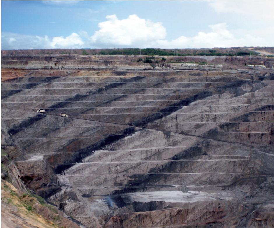
Figure 5.10: Several meters thick hard coal seams in semisteepl stratification in the surface mine Panian on Semirara Island, the greatest surface mine of the Philippines.
