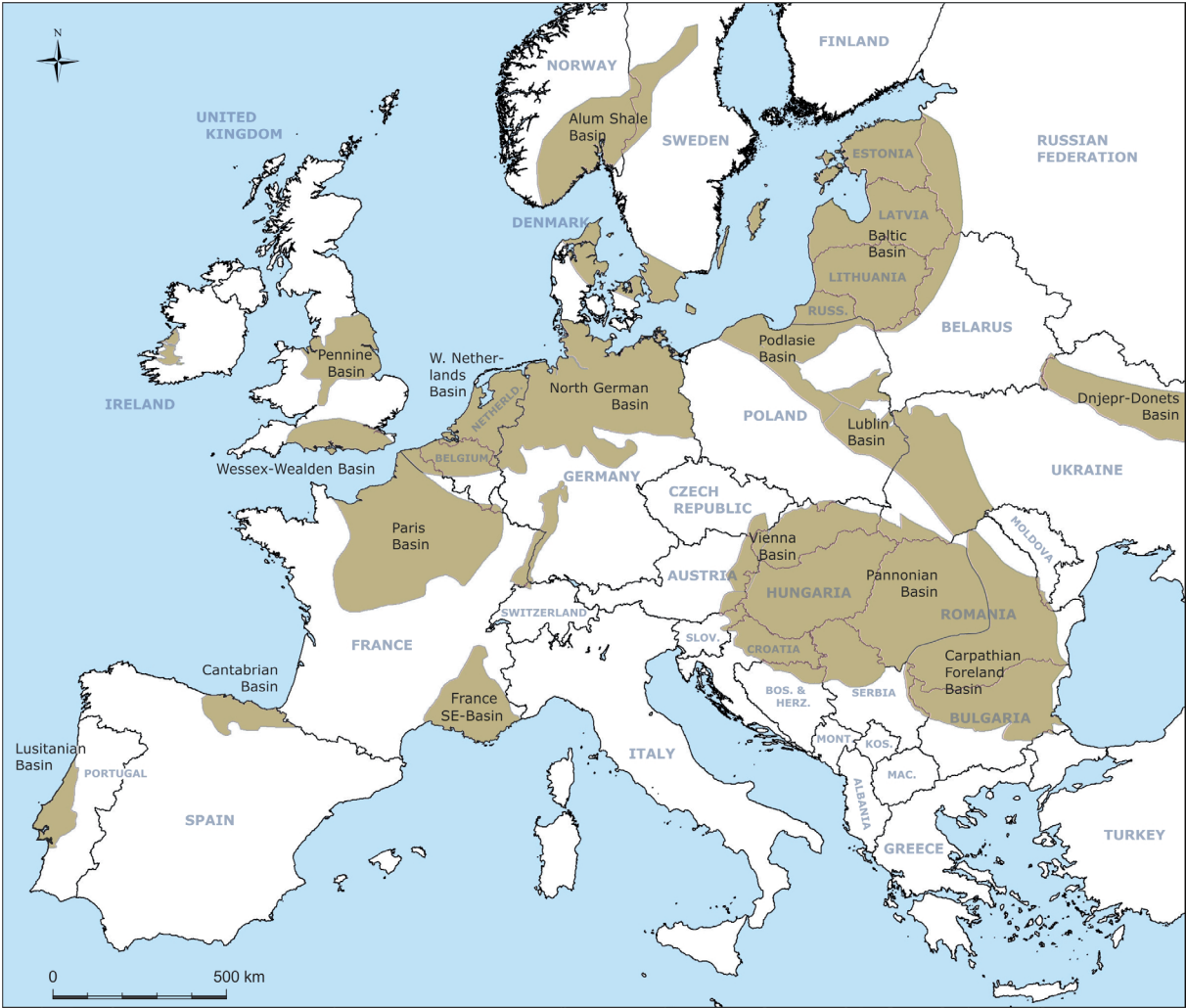
Fig. 13: Schematic diagram of the geological basins with possible light tight oil and shale gas potential in Europe.
