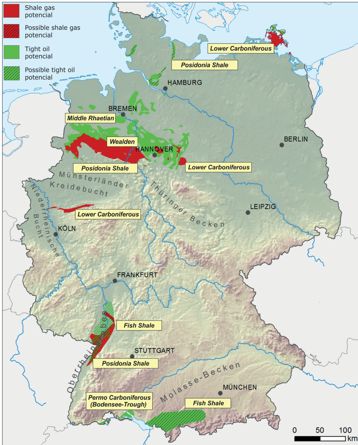
Figure 35: Overview of the areas with shale oil or shale gas potential including the name of the shale formation in each case: hatched areas: areas with possible shale oil or shale gas potential; the potential within these areas only exists in smaller sub-zones which cannot be localised more precisely by the study (BGR 2016b).
