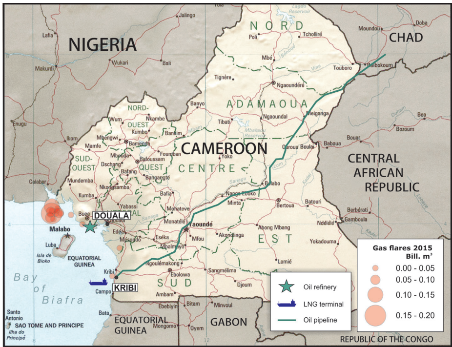
Figure: 4-7: Gas flaring and oil infrastructure in Cameroon.
