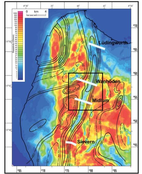
Apparent resistivity map ( $f=1840$  Hz) derived from helicopter electro-magnetic survey (HEM) after Siemon et al. (2004). The contour lines show the base of Quaternary in meter b.s.l. (Kuster and Meyer, 1995). The seismic profiles are marked in white and the SkyTEM survey by a black rectangle.
