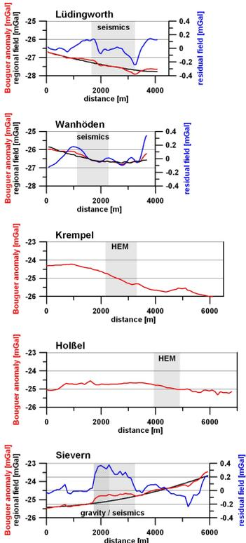
The change in the valley fill is reflected by the Bouguer anomaly. Positive, in general, it is overcompensated by a near-surface clay (Lüdingworth) or a moor (Wanhöden).
