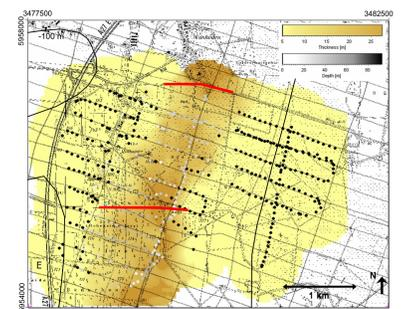
Based on SkyTEM data (Aarhus University) the Lauenburger clay is roughly 15 - 30 m thick (brownish colours) and 40 - 60 m deep in the Midlum/Wanhöden area. The red lines mark the buried valley in the seismic lines. The black lines denote the 100 m depth contour after Kuster and Meyer (1995).
