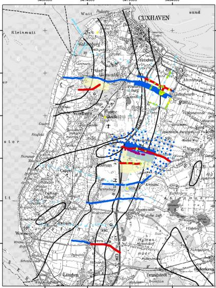
Legend: Reflection seismic (—), Gravimetry (●), SkyTEM (—), TEM (●), Vertical electric sounding (▲), CPT (●), Well logging (▲).
