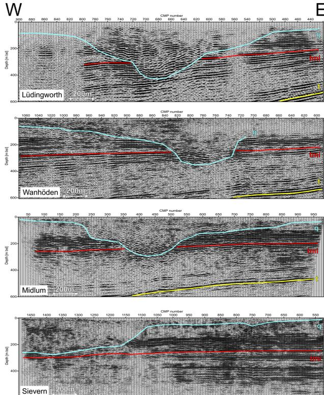
Seismic profiles across the Cuxhavener Rinne from north (Lüdingworth) to south (Sievern). The coloured lines show the interpreted base of Tertiary (—), the base of Miocene (—) and the base of Quaternary (—). Note the flattening of the buried valley and the varying shape of its shoulders.
