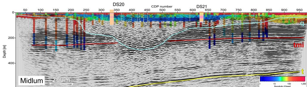
Above: At Midlum the covering clay layer shows up clearly in the SkyTEM data (blue). It is marked in the seismic section by a strong reflector (e.g. DS21). The valley is narrower than
