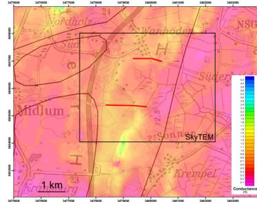
HEM conductivity map for 25 m depth. Only thin clay layers are found above the buried valley (orange colours).
