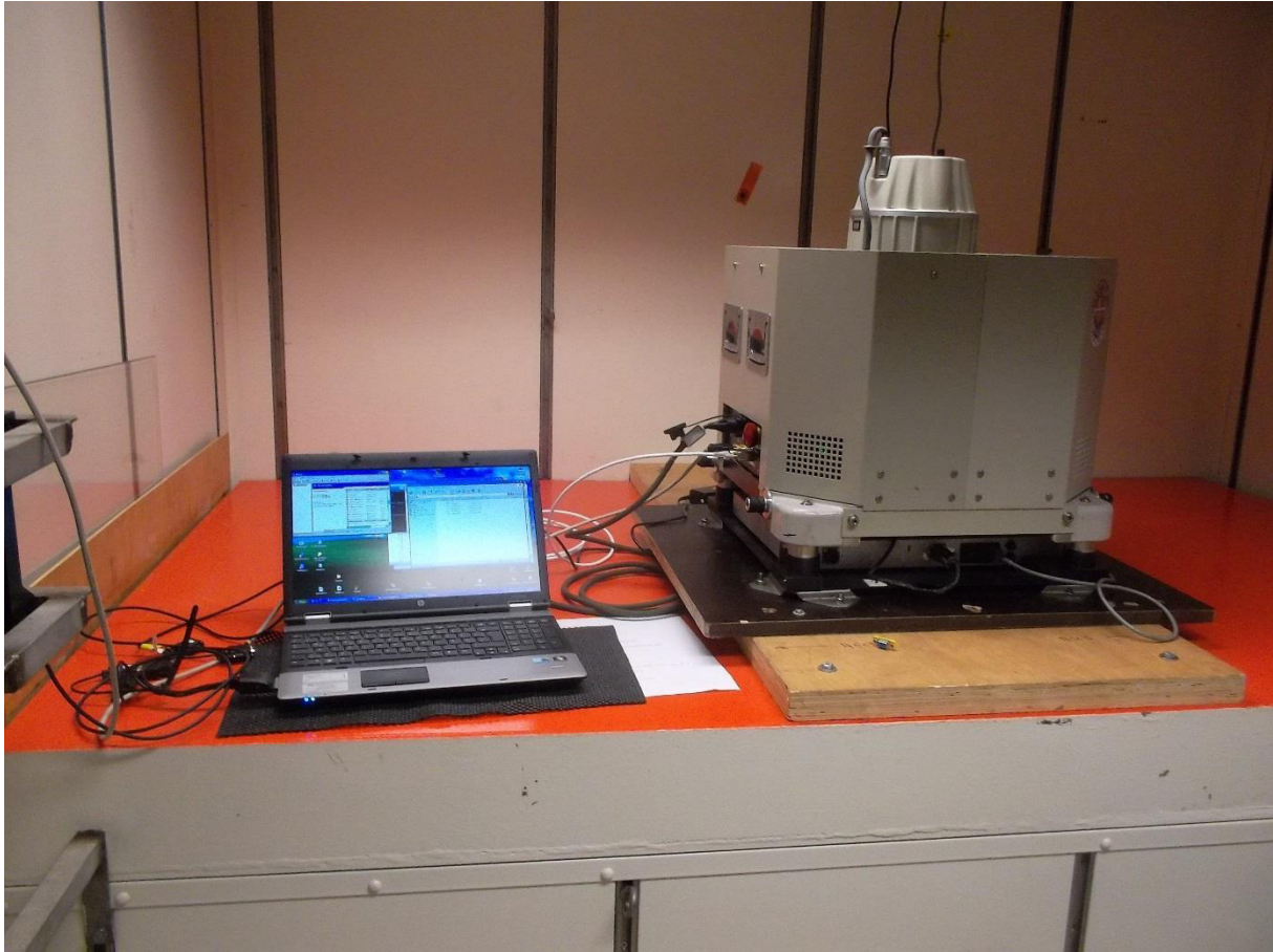
Figure 5.1 2: KSS32-M gravimeter system in the gravimeter lab of RV Merian.
