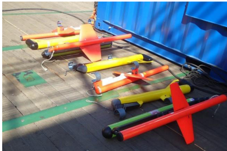
Figure 5.4. 4: Streamer devices: DigiBirds for depth control and compass heading (red), CMX units for acoustic measurements (yellow), and recovery system (green).
