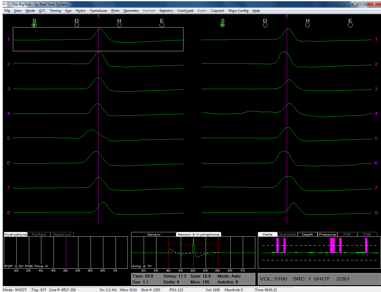
Figure 5.4 2: Shot timing of all 16 G-guns for BigShot.
