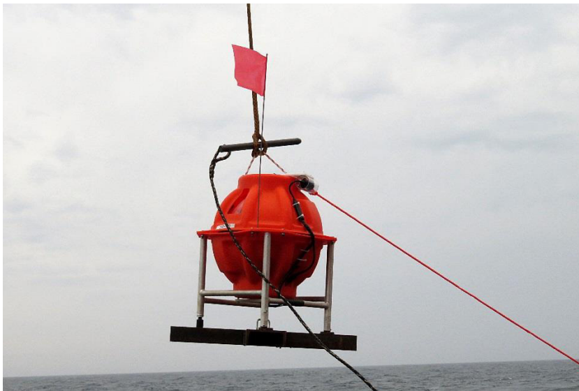
Figure 5.5 1: Sercel MicroOBS_Plus during deployment along line BGR17-2R1 (photo: Thomas Funck).
