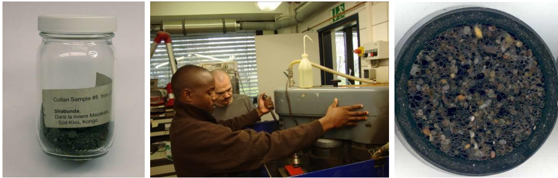
Figure 2: Left – Typical AFP mineral concentrate sample (ca. 50 g; diameter of flask = 4 cm); Center – Grinding machine used to prepare mounted AFP sample for polishing. Right – Polished section of sample for AFP analysis.
