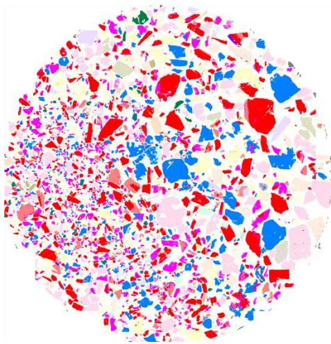
Fig. 8: Left - Automated mineralogy image of a polished section prepared from a cassiterite-coltan ore concentrate; Right – Legend and mineralogical composition
