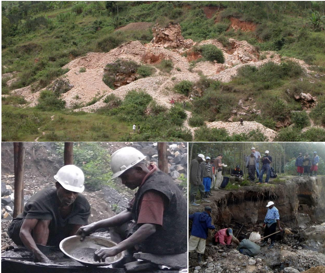
Figure 1: Top – Pegmatite-related cassiterite-coltan mine site in the Great Lakes region (Gatumba, Rwanda) of typical size (few dozens of meters in diameter; note artisanal miners for scale); the commonly small spatial dimension of individual mine sites is one of the key factors for the high spatial resolution of the AFP method. Lower left – mineral pre-concentrate produced on site by artisanal miners through panning; this type of concentrate represents the ideal AFP sampling material (for reference database construction). Lower right – Joint BGR-GMD AFP sampling in Rwanda (note that most persons on the photograph are artisanal miners/mining company employees; a single person is generally sufficient to carry out sampling).
