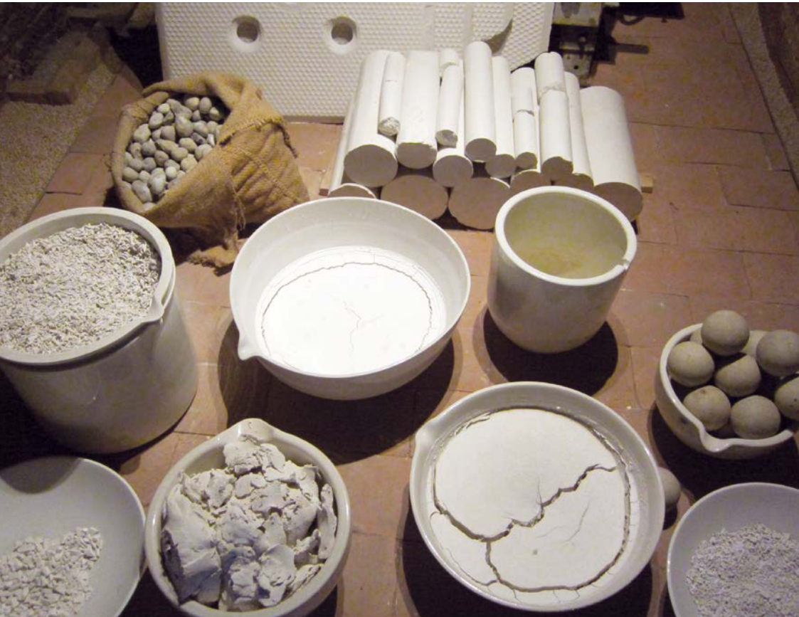
Figure: 4: Before application in the final stage, feldspar raw material passes through various intermediate processing steps from filter cake to ceramic masses (Photo: BGR).
