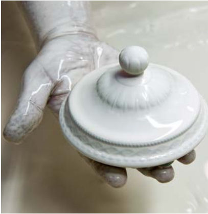
Figure 5: Application of glaze on ceramic product. (Photo: with kind permission of KPM Berlin).
