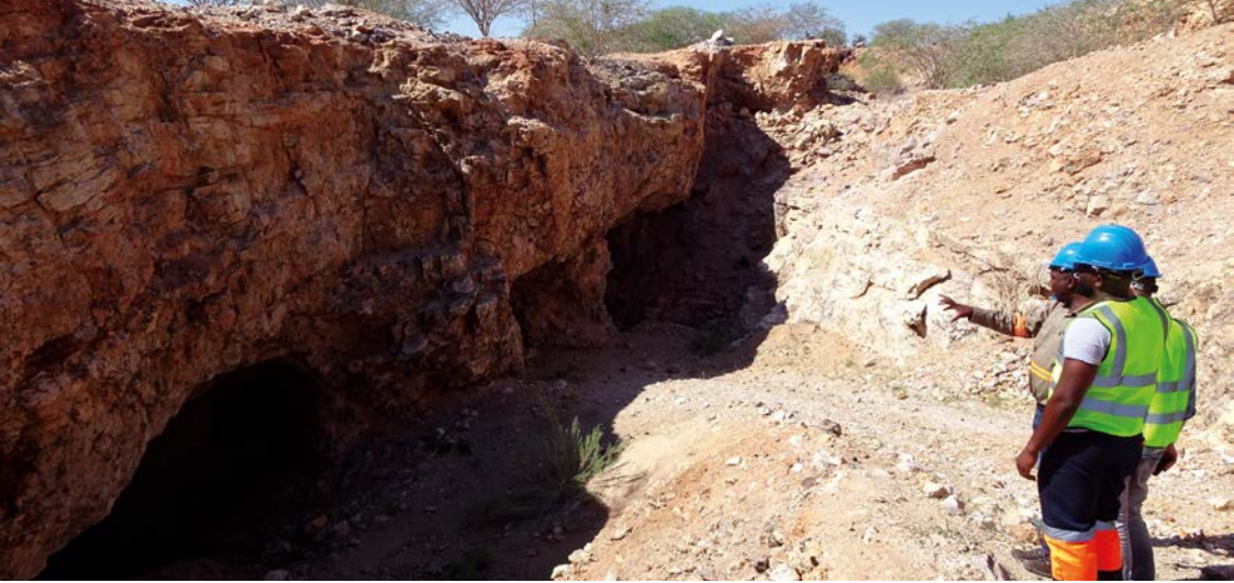
Figure 16: Remnants of room and pillar mining at historic mine site at Rubicon pegmatite (Photo: BGR-GSN-Project 2019, with kind permission of Lepidico Chemicals Namibia (Pty) Ltd.).
