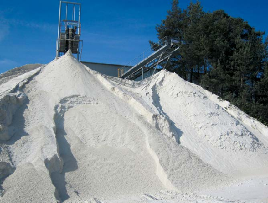
Figure 10: Feldspar raw material requires processing before introduction to the market. Customers are supplied with milled feldspar of different mesh sizes (Photo: BGR).
