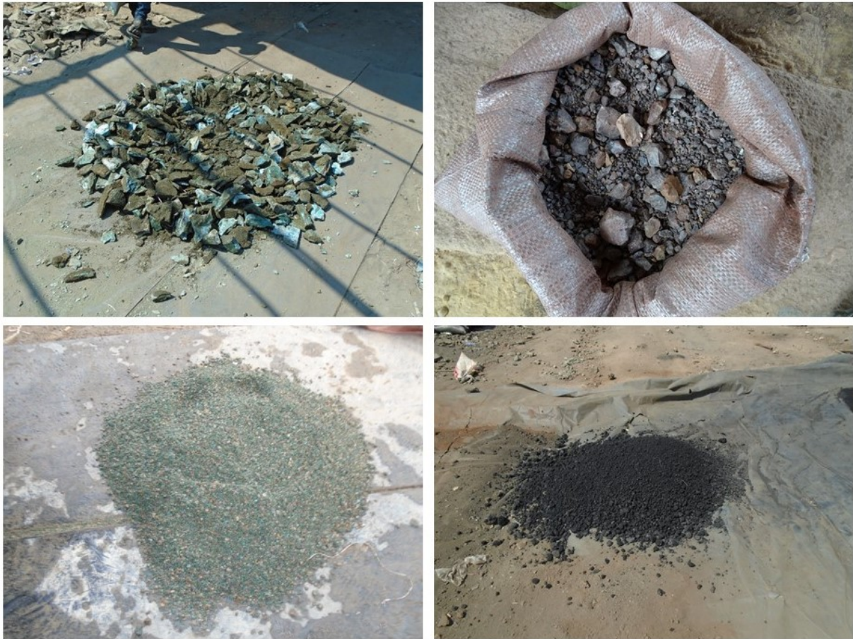
Figure 15. Copper ore (left) already crushed and cobalt ore milled (lower right) or unprocessed and ready for transport (upper right).
