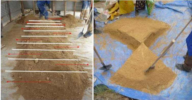
Figure 3: Workers are splitting the bulk samples representatively after homogenization. Left: riffle splitting, half of the sample goes to the right, the other half to the left; Right: Quartering, by quartering the pile and combining the quarters opposite to each other, two representative samples are formed
