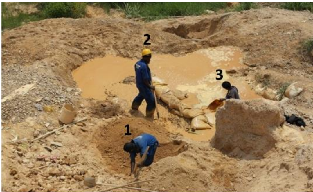
Figure 5: Circuit ground sluicing with material feeding (1), moving of the material in the opposite direction of the water flow (2) and supply of the water stream (3)
