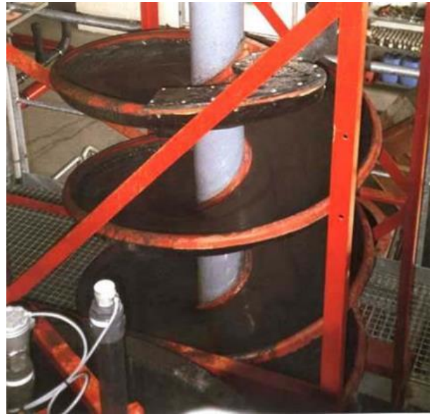
Figure 12: Spiral concentrator fed with liquid pulp.
