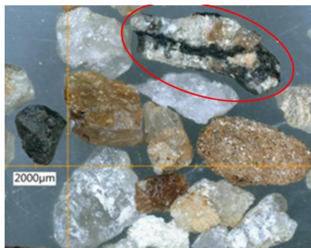
Figure 20: Picture of reflected-light microscopy of the grain-size fraction 2 mm to 5 mm of ROM 2
