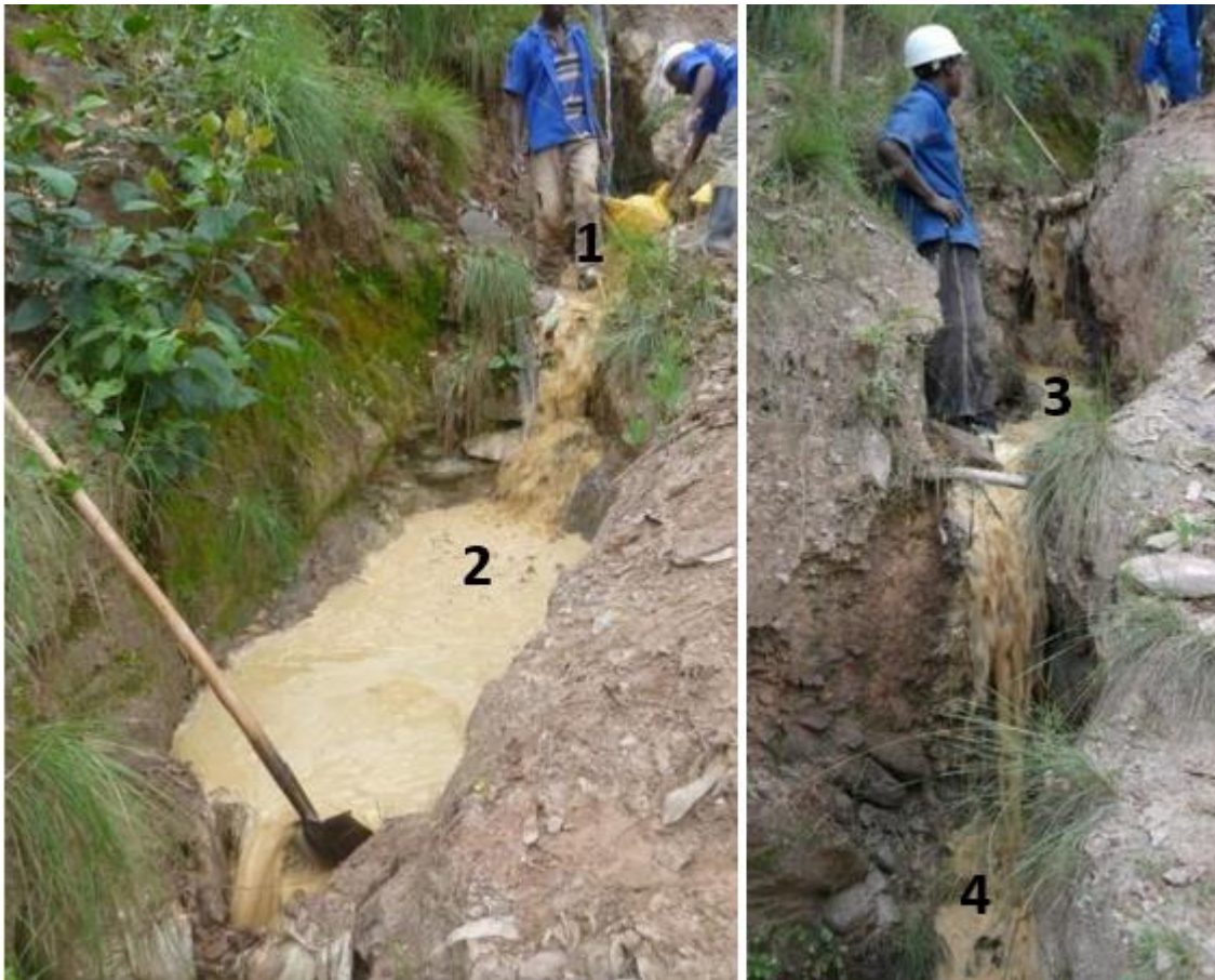
Figure 6: Linear ground sluicing. (1) Feeding of the ROM and water; (2) first concentration stage and narrowing of water stream/reducing water mass and velocity with a shovel; (3) second concentration stage; (4) possible third concentration stage.
