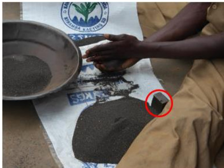
Figure 9: Artisanal magnetic separation of a mixed concentrate with manual magnet (red circle)
