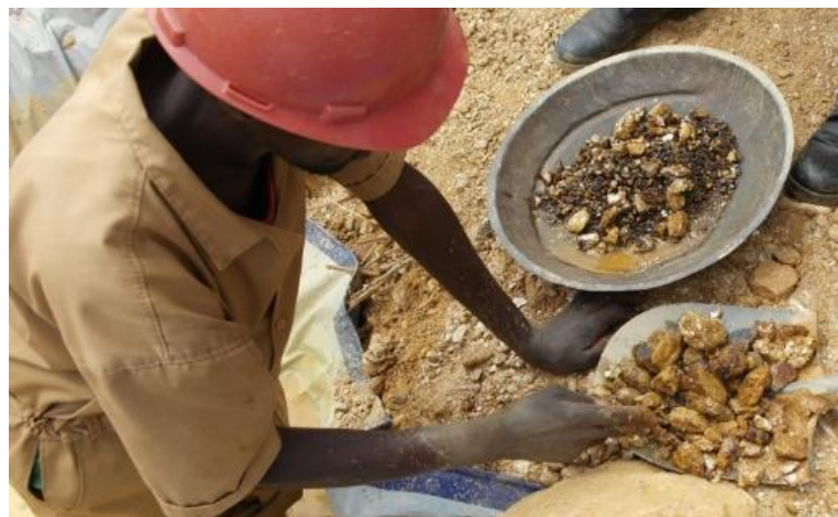
Figure 7: Visual evaluation and handpicking of coarse rocks after panning
