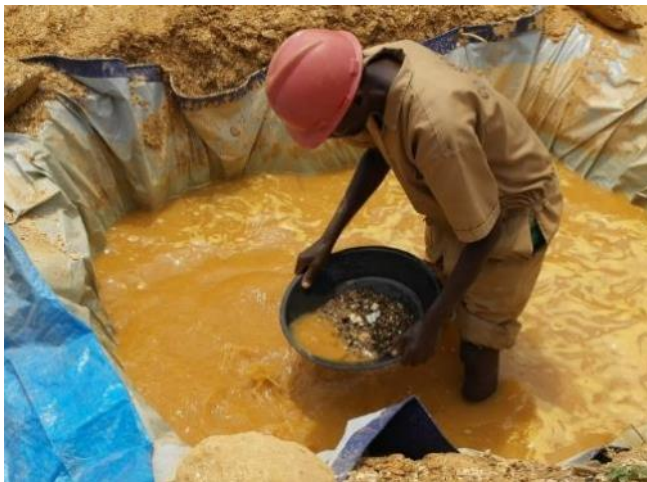
Figure 4: Panning process in prepared washing pond
