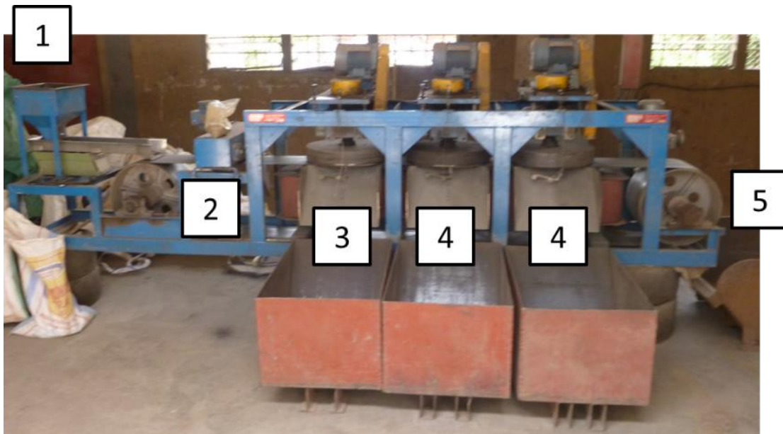
Figure 16: Magnetic separator with multiple electromagnets of variable magnetic intensity. The feed section is at (1) where the material is put on a vibratory feeder. At (2) the high magnetic fraction is separated by a low energy magnetic field. At (3) another high magnetic fraction is separated. At (4) low magnetic materials are removed and at (5) nonmagnetic material remains.
