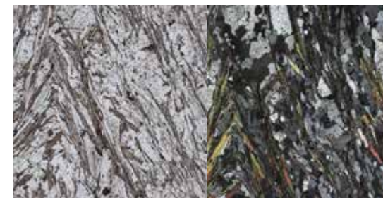
Thin section of a folded mica schist from Spitsbergen consisting of biotite, muscovite and quartz. View in plane-polarised light (left) and with crossed polarisers (right).
