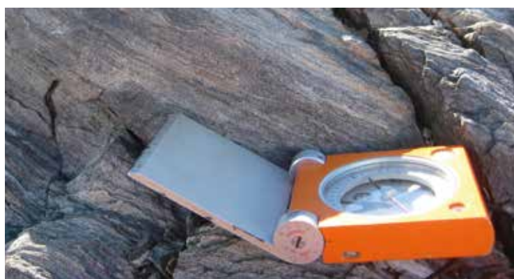
Measuring the lineation of a gneiss with a geological compass in Dronning Maud Land, East Antarctica.
