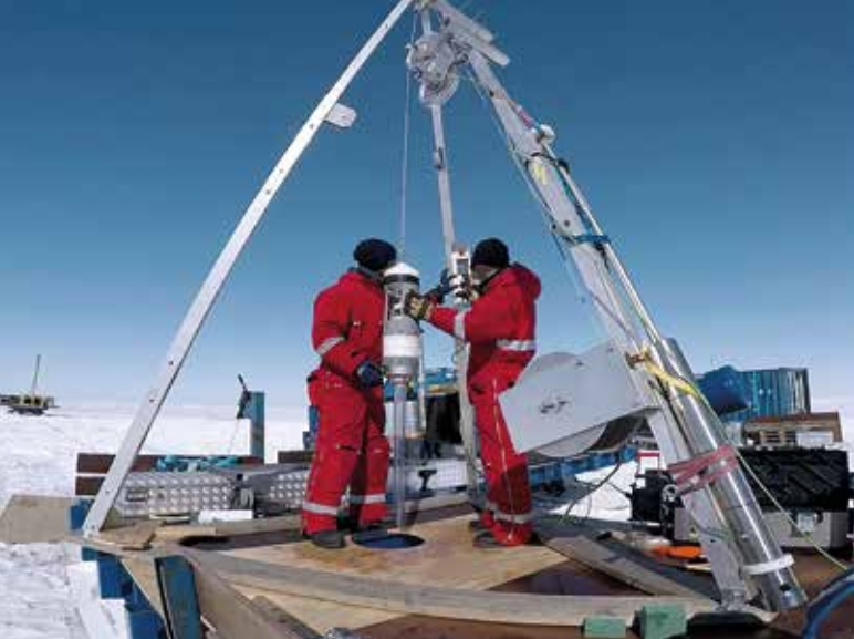
Sampling with a gravity corer during the Sub-EIS-Obs II expedition on the Ekström Ice Shelf.
