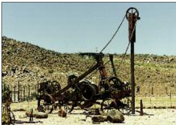
Old drilling machine for groundwater boreholes
