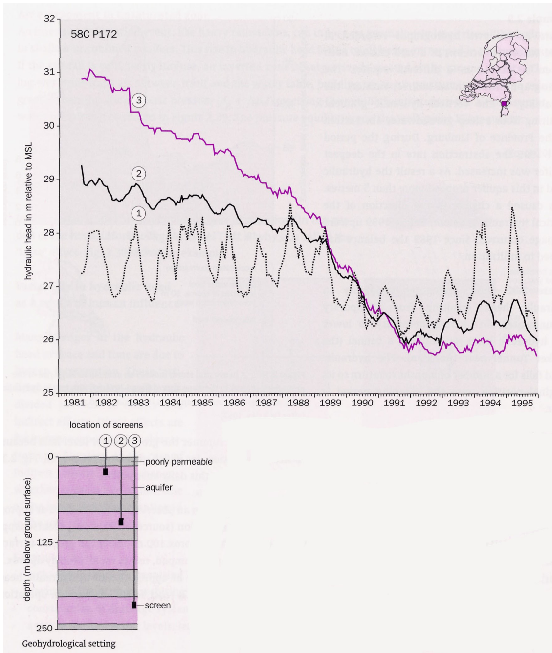
Figure 14: Hydrographs of a Cluster Well in the Roer Graben near Limburg/The Netherlands showing Response to High Groundwater Abstraction in Deepest Aquifer (from Van BRACHT 2001)
