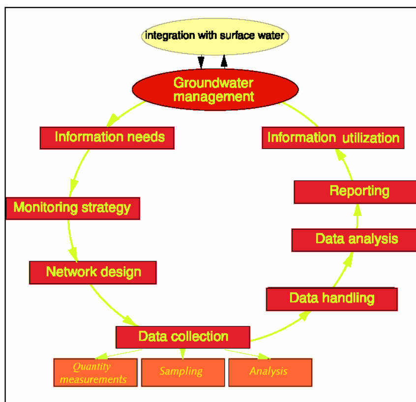
Figure 1: Components of Groundwater Monitoring
