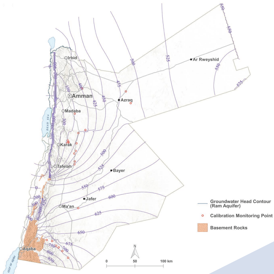
79 Groundwater contours for the predevelopment conditions in the Ram/Disi aquifer
