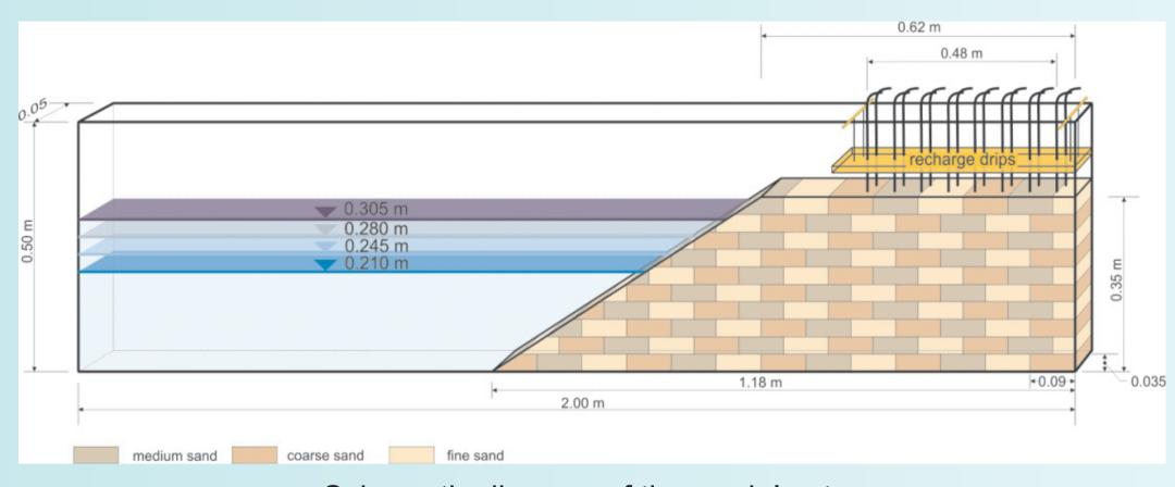
Schematic diagram of the model setup
