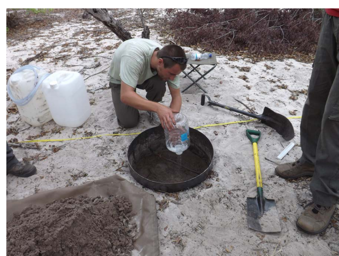
Fig. 1: Application of deuterated water at 25 cm depth
