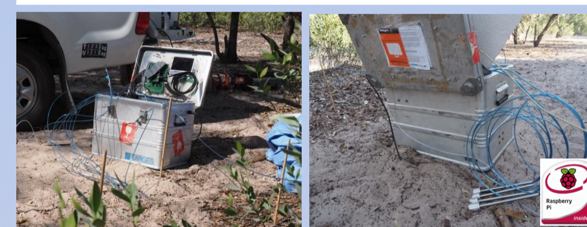
Fig. 4: Custom built soil gas sampler using raspberry pi....
