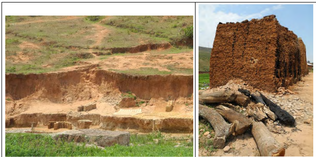
Figure 4.8: Left: thick soils in valley bottoms are used for the production of bricks. Right: Simple oven for the brick production. Both locations situated east of Gitega.
