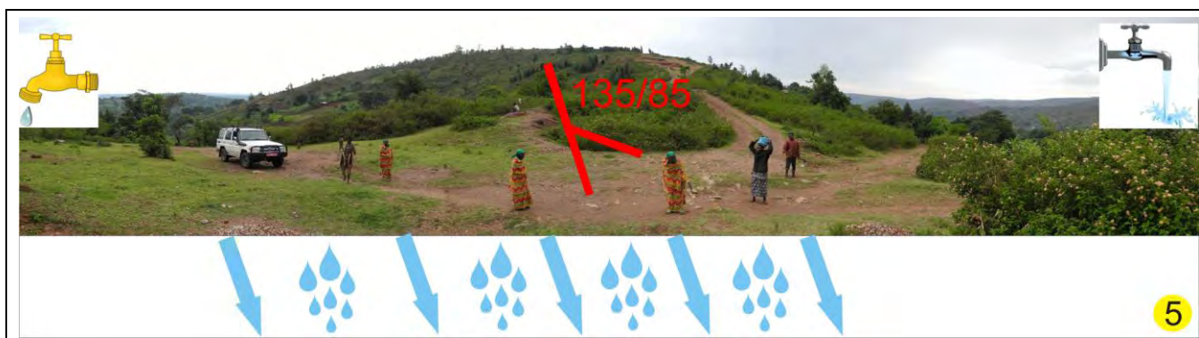
Figure 6.18: View from 320° to 110° (WP 21). A lineament of Category 2 is divided by a ridge. Schist foliation is dipping steep (85°) to SE. A well in the NW supplies only little- while a well in the SE delivers plenty of water. The most probable reason is additional groundwater contribution by open foliation in this area.
