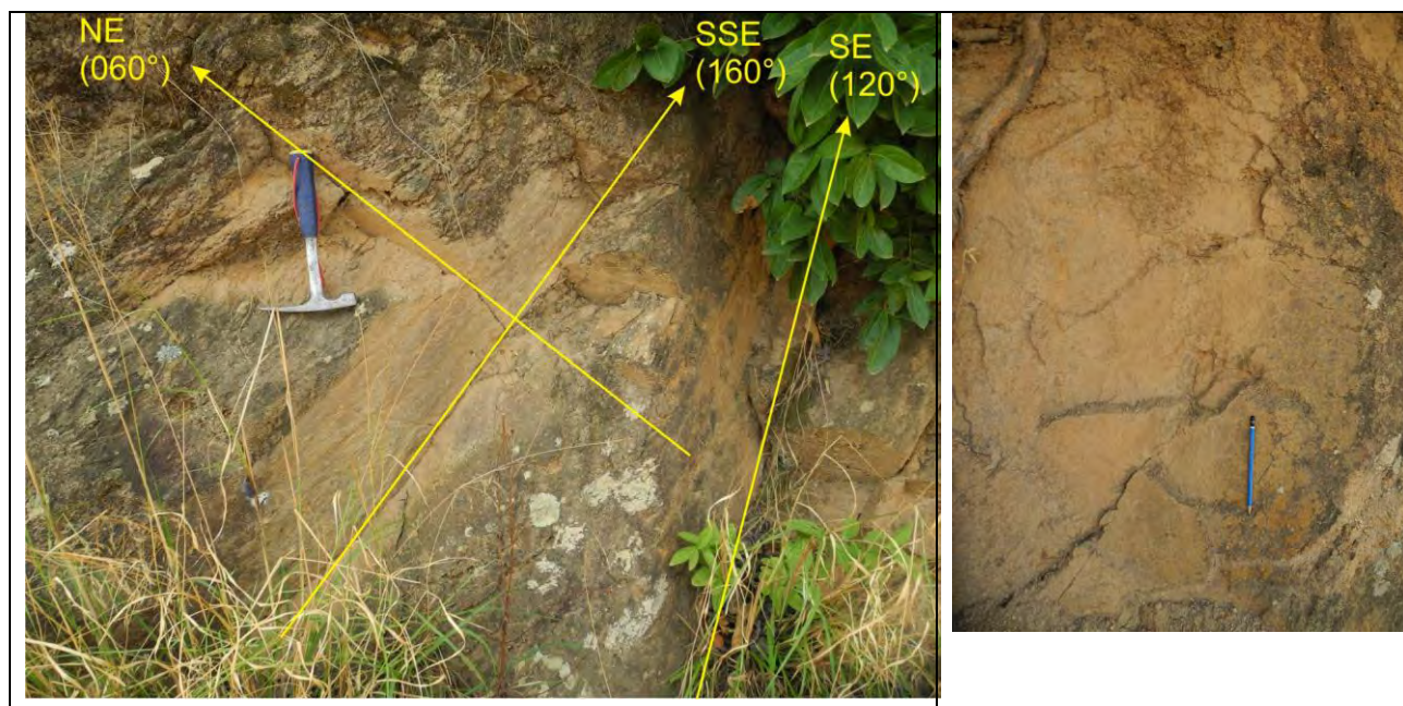
Figure 5.5: Left: (WP 85) Outcrop showing different joint planes with corresponding lineament directions at a small scale. Right: (WP 84) Tear-off edges show an upward-directed relative-movement of a former hanging wall.
