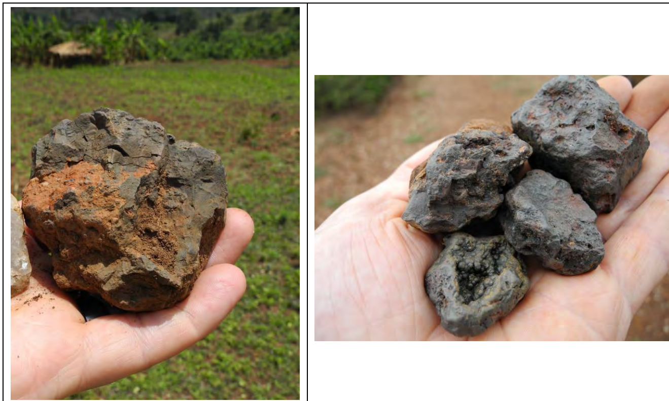
Figure 4.10: Left: thick iron oxide crust (WP 29). Right: Iron concretions (WP 21) genesis by intensive tropical alteration. Both locations are situated north of Kirundo.
