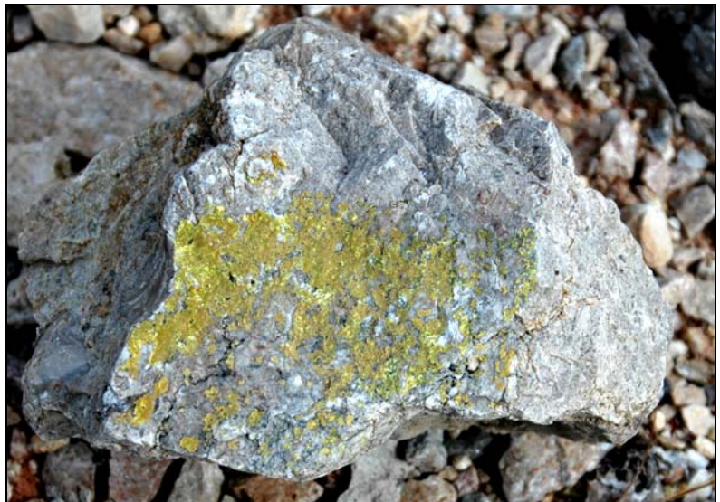
Figure 4. Uranium ore as collected on a waste rock dump. The original uranium mineral Pitchblende is oxidized to Carnotite and Tyuyamunnite .
