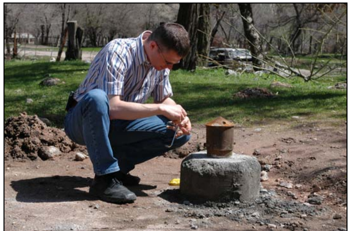
Figure 19: Groundwater-monitoring-well downstream of tailings impoundment No. 6.
