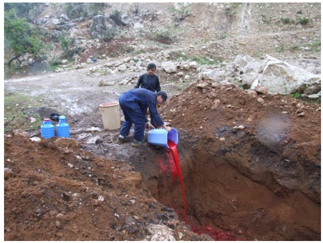
Figure 2-2 Amidorhodamin G Injection and Flushing in Abu Mizane pit hole on April 22 nd , 2010 (15:59)
