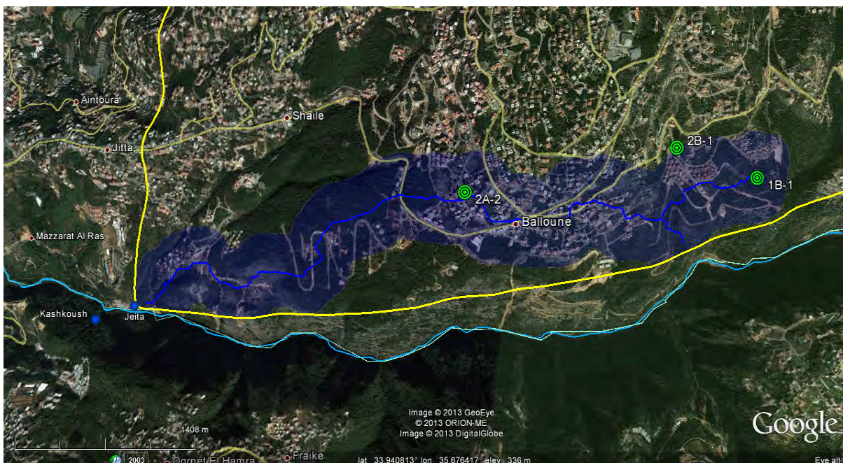
Figure 13: Buffer zone of 250 m from the center line of Jeita cave, defining groundwater protection zone 2A according to very high risk of infiltration
