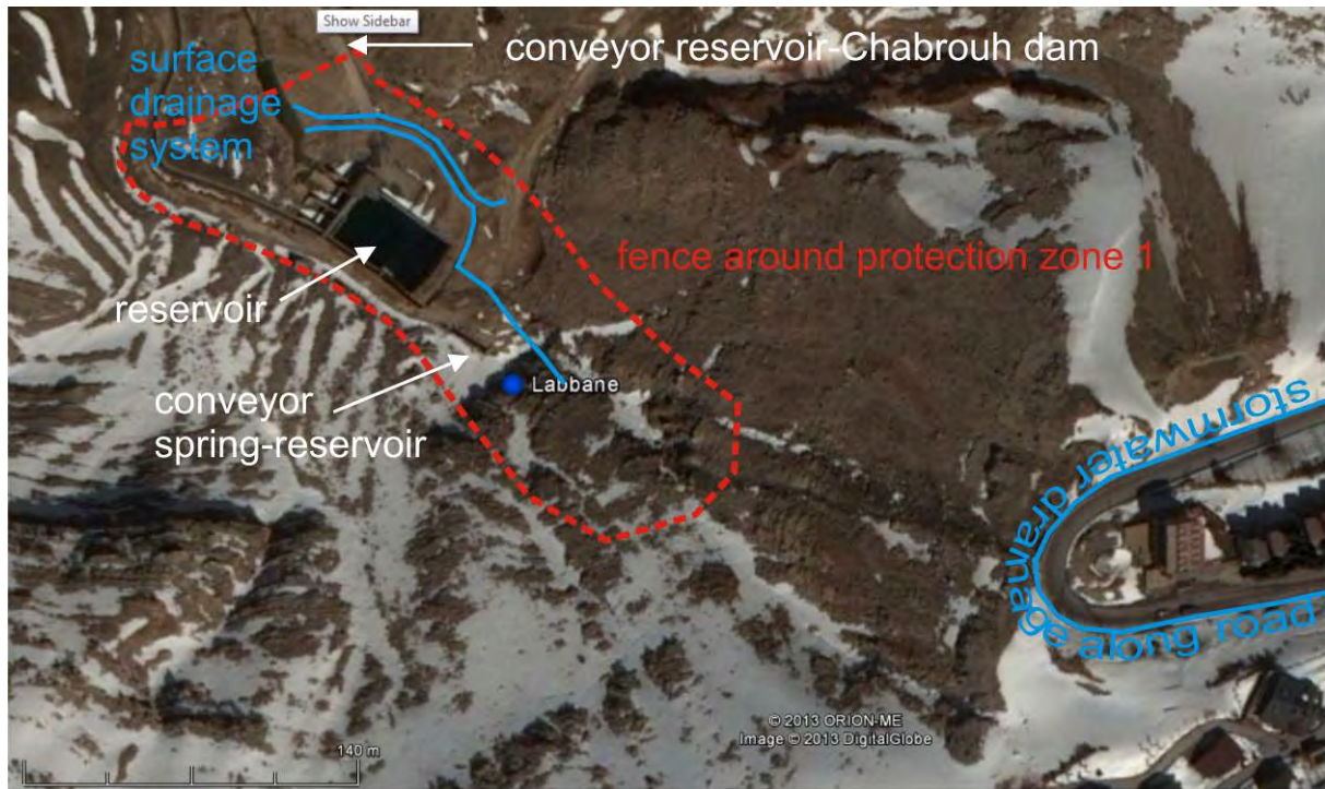
Figure 31: Protection Zone 1 of Labbane Spring with proposed fence and surface drainage systems
