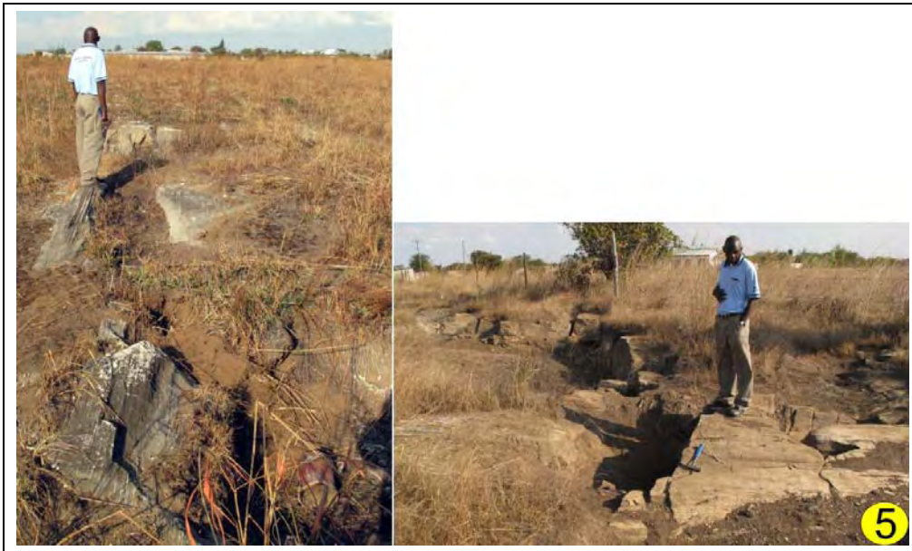
Figure 51: Soil-filled karst holes between steep layers of Lusaka Dolomite in development area (WP 008).
