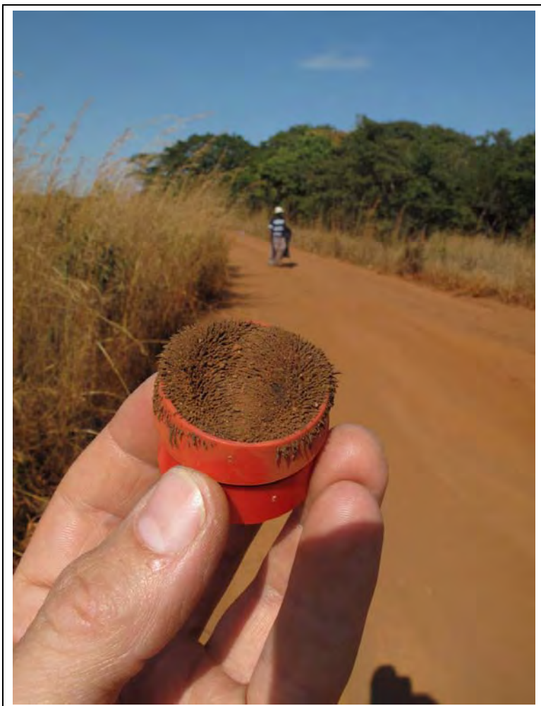
Figure 30: Dispersed magnetite in plinthic soil sticking to a magnet (WP 034).
