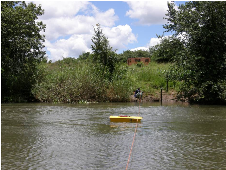
Fig. 5 Discharge measurement with OTT QLiner
