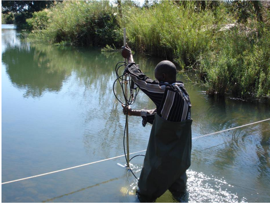
Fig. 3 Discharge measurement with OTT ADC
