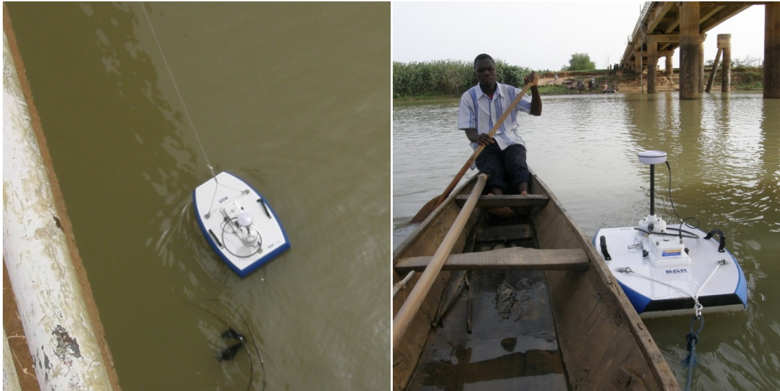
Fig. 2 Discharge measurement at Malanville from bridge and pirogue
