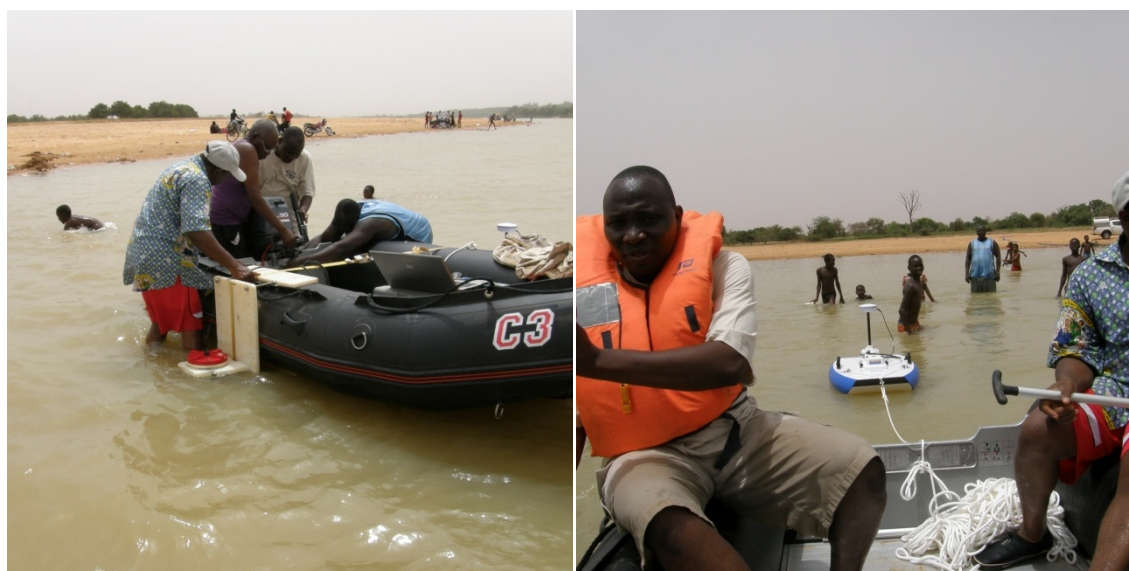
Fig. 10 Discharge measurement with both ADCP (left ABN instrument, right BGR instrument)
