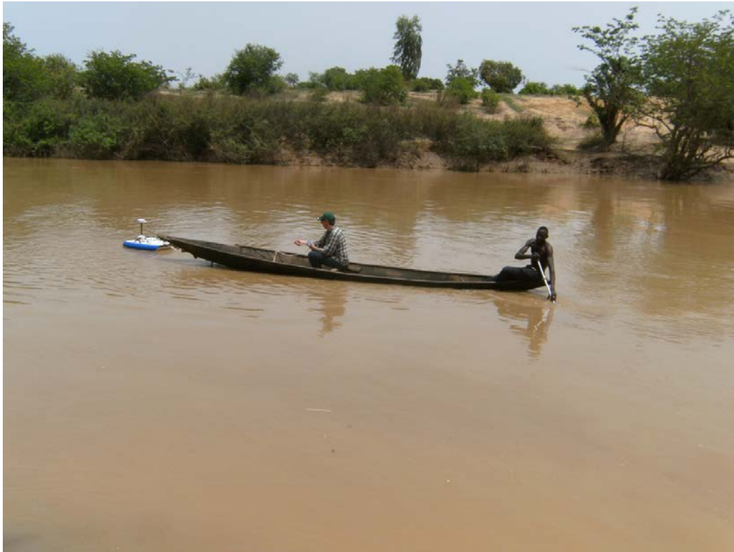
Fig. 16 Discharge measurement at Sota River at Malanville
