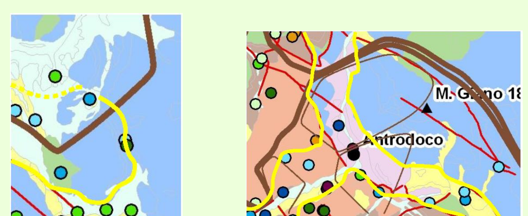
Fig. 8 – A detailed comparison between the obtained contour lines and the EC values distribution in the map has allowed to undertake the final tracing of hydrogeological boundaries (and left) to understand in which sectors the hydrogeological boundaries are actually buried under the alluvial cover, and thus evidenced with an appropriate symbol (dotted yellow line). In sectors where control points are lacking (e.g., M. Giano area) the final tracing of the hydrogeological boundaries may be very different from the computer assisted contour line drawing process results (right).
